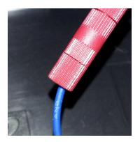
Tighten the end and pull gently on the wire to verify it is secure.
