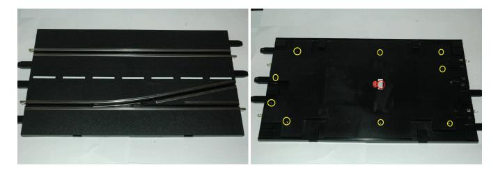
7. Place the section so that the IR sensor (with blue/yellow wires) is at bottom right. The numbers on the right side of the picture help identify each of the track rails. The factory red (+) wire may be located in rail #1 or #3 and either position is acceptable. If the factory black (-) wire is in rail #2, move it to rail #4 as shown below.
