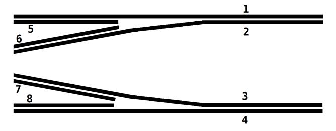
Disconnect LG wire from #1, move to #8. (does not apply to Right lane changers) Disconnect LG wire from #4, move to #5. (does not apply to Left lane changers) Stock LG harness will need wire(s) extended about 5cm (2") to reach.
