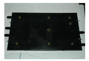
3. Isolate the inside rail of the destination lane by removing the jumper wire as shown. It is <u>usually</u> a black wire. On curved lane changers that have a long and short half for each jumper, remove only the short black half.
