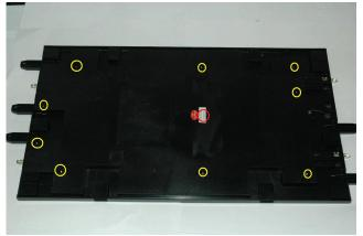
7. Place the section so that the IR sensor (with blue/yellow wires) is at top right. The numbers on the right side of the picture help identify each of the track rails. The factory black (-) wire may be located rail #2 or #4 and either position is acceptable. The factory red (+) wire must go to rail #1. If in rail #3 as shown below, move it to rail #1.
