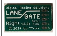
The DRS Lane Gate "Right" chip is for D124/D132 lane changers where cars can move from the left lane to the right lane only. That includes models #30345 Straight Type, #30362 Left Curve - In to Out, and #30365 Right Curve - Out to In
