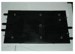
3. Isolate the inside rail of the destination lane by removing the jumper wire as shown. It is <u>usually</u> a red wire. On curved lane changers that have a long and short half for each jumper, remove only the short red half.
